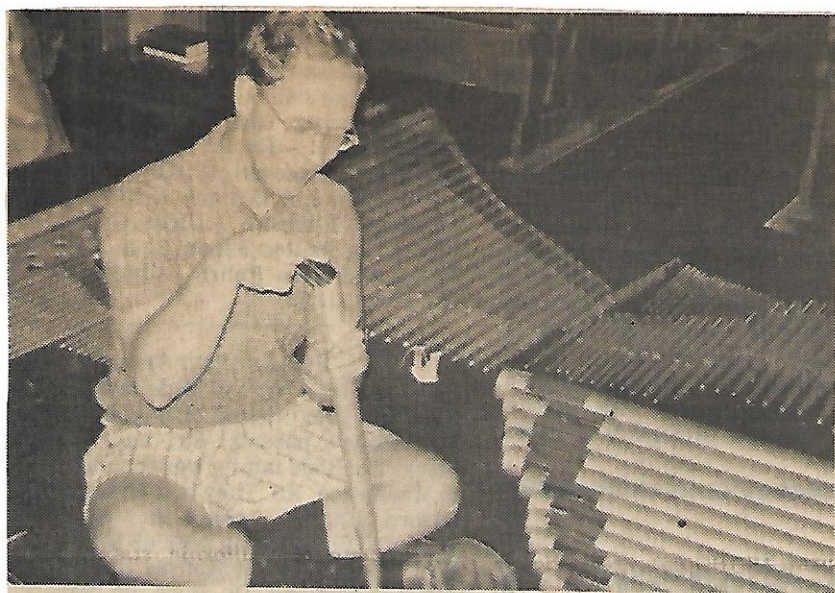
Michel Quimby is shown slipping a metal sleeve over the end of a metal pipe. After the pipe is placed in the organ it is necessary to adjust each sleeve on each pipe to reach the desired note. A pipe organ has an advantage over a stringed instrument, such as a piano, in that, once properly adjusted, it holds a tone for a prolonged length of time.
