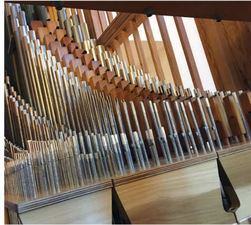
Great pipes at Southern Shores (L to R): Mixture III, 2' Fifteenth, 4' Octave, 8' Dulciana, 8' Hohlflute, and 8' Open Diapason (photo credit Steve Blackstock)
