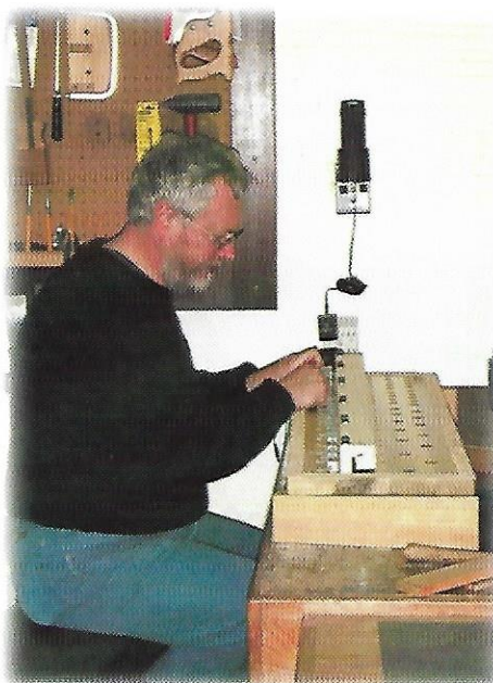
John Wiring the Magnets on Action Board
