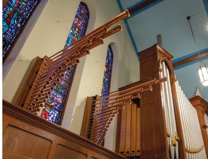
The new 8' Trompette-en-Chamade, with vertically oriented chests, and close-up view of new casework and facade pipes on the right side, in front of the Great and Solo divisions.
